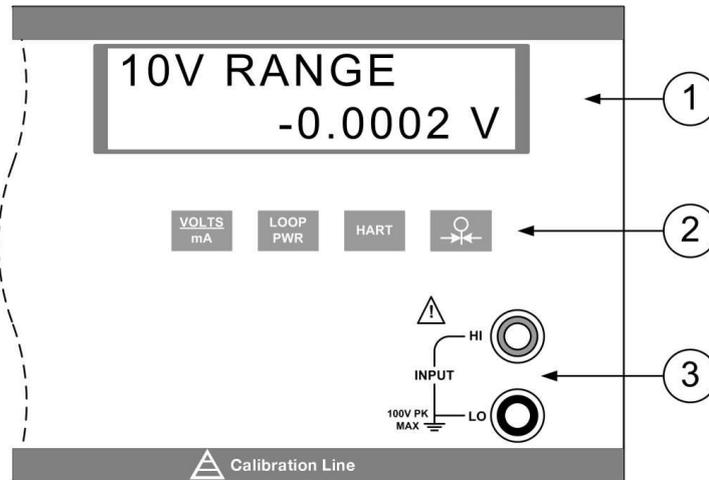
**Figure 4 - Isolated Input Display, Controls, and Terminals**
