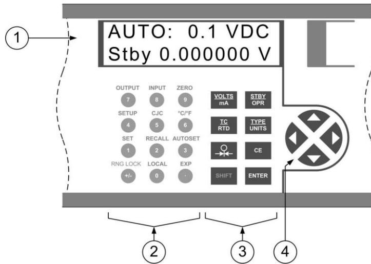
Figure 3 - Primary Input/Output Display and Controls
