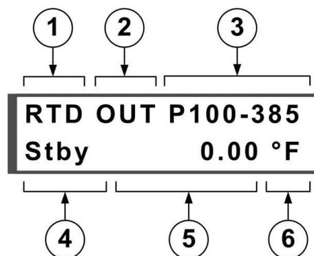
Figure 7 - Primary Thermocouple and RTD Display Layout
